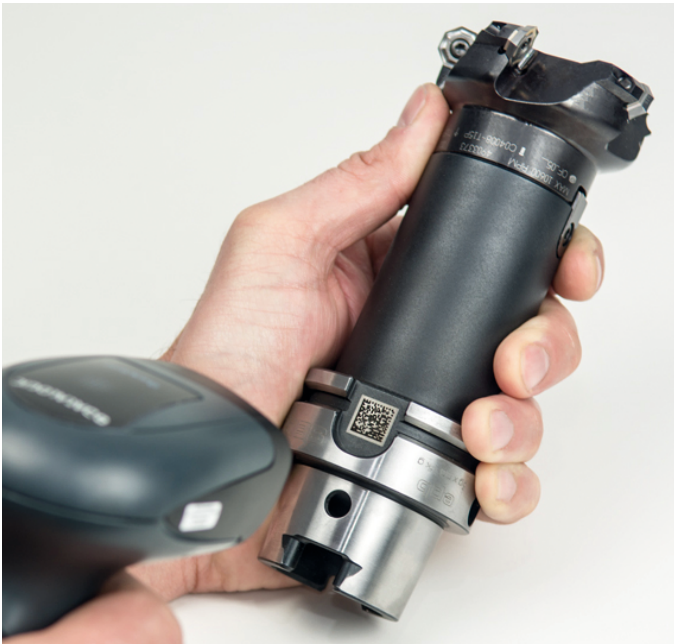
Tool assemblies are now clearly identifiable, and their data can be transferred to the machine via a scan.
