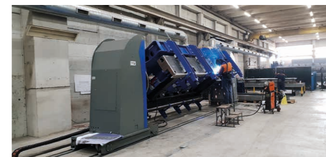
View of the production line in operation with clamping device featuring lifting/rotary axes
